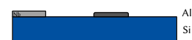
Fig. 6.12: Outline of the pillars fabrication process. The starting point is a wafer with Niobium (Nb) structures (light grey rectangle) fabricated in the previous stage. For more details, refer to the main text.
